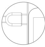
Only use the charging cable provided in the package for charging. In the event that the included cable is lost, ensure that the pen scanner is charged using a power adapter compliant with DC 5V--2A specifications (USB Type-A to USB Type-C).
